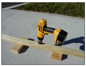
Stack lattice pieces, and drill 1/4" holes starting in the center and working your way to the edge with a hole drilled at 12" from the center hole.
