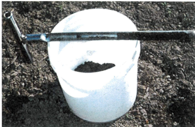
Figure 2: Typical soil probe and a bucket that you can use to collect the “Core” samples.
