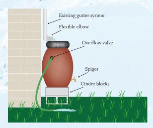
Composed of a large container or barrel, a piece of vinyl hose, PVC couplings, a screen grate to keep out debris and insects, a faucet, and pieces of gutter, all from the local hardware store. Add the use of a few household tools and 30 minutes, and a rain barrel is relatively easy and economical to construct and can be used with any residential gutter system.
