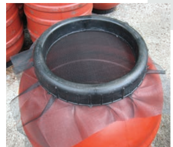
For barrels with a removable lid, unscrew the retainer ring and separate it from the inner lid, place screen over barrel opening, replace just the retainer ring to hold the screen in place, and trim excess screen material around the outside of retainer ring.
