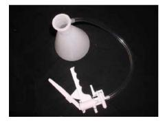
**Step 3:** Assemble the filter funnel. Grasp the cup base by the rubber stopper and gently twist it downward into the mouth of the filtering flask.
