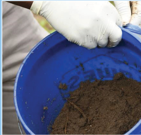
Thoroughly mix the 15–20 core samples in a nonmetal bucket. Credits: T. R. Weeks, UF/IFAS
