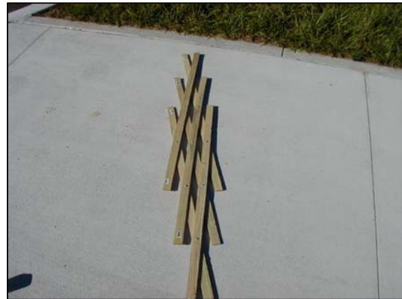
With the bolts, nuts and washers in place, the grid can be folded up for storage when garden is shut down.
