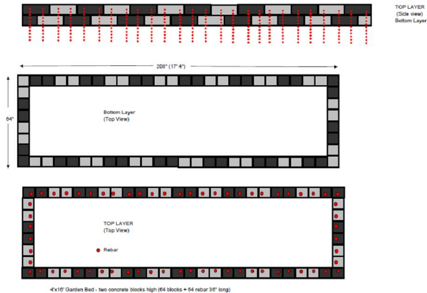
Raised Beds (16" height) from Concrete Blocks (Rebar for strength)
