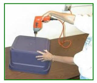
2. Drill ventilation holes about  $1 - 1 \frac{1}{2}$  inches apart on each side of all the containers near the top edge using the 1/16 inch bit. Also drill about 30 small holes in the top of **one** of the lids.
