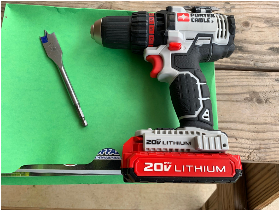
We used a 13/16" drill bit to cut the overflow and spigot holes.
