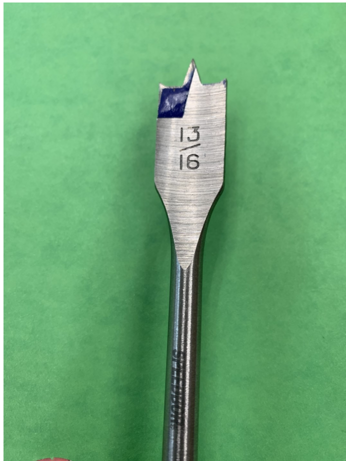
We used a 13/16" drill bit to cut the overflow and spigot holes.
