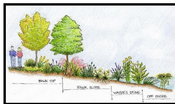
Figure 1 Illustration of stormwater pond planting zones along a moderate to gentle slope. Credit: Gail Hansen, UF/IFAS
